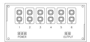
Rear panel of a SWT-11006-...x-Indicator-special with a 6 standard jack inserts in correct calibration. Power connection (L, N, earth) with screw terminals, output, screw terminals.
